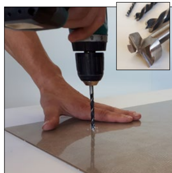
Corner relief drilling using a wood drill with a centring tip
